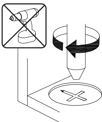
**EN**\_Turn cam lock clockwise to tighten.
