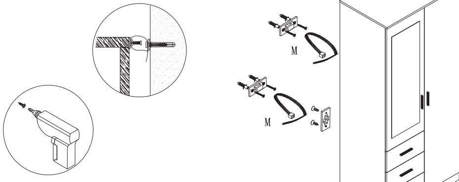
**EN**\_If it is a solid wall, please use expansion and self-tapping screws, if it is a wooden wall, only use self-tapping screws, please do not overtighten the screws
