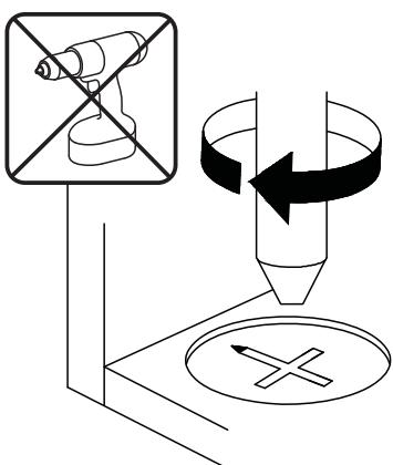
**EN**\_Turn cam lock clockwise to tighten.
