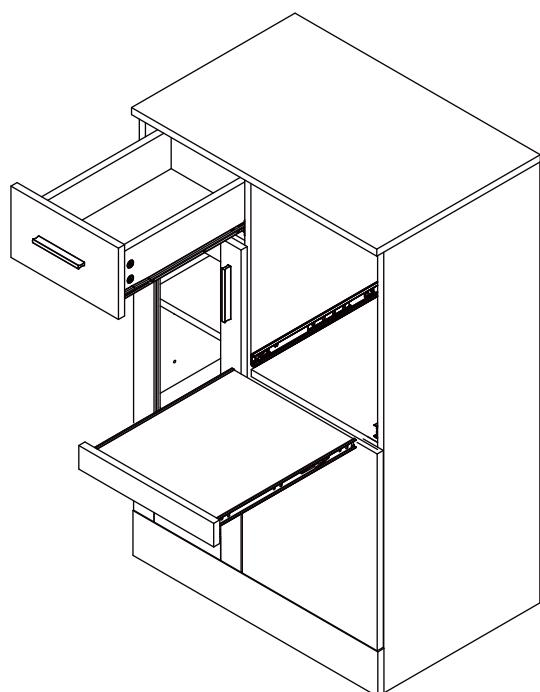
**EN** Be careful to push in the board when the both sides slide way been aligned.
