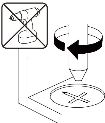
**EN**\_Turn cam lock clockwise to tighten.
