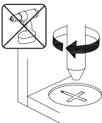
**EN** Turn cam lock clockwise to tighten.
