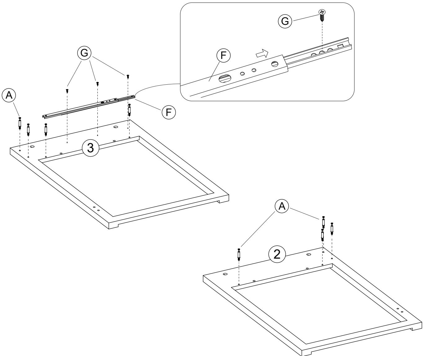
**EN** Please find the exact hole for installation, otherwise it will be misaligned. The screws on the drawer slide must be leveled , otherwise it will affect the smoothness of the drawer.
