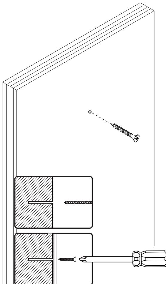
**EN** If it is a solid wall, please use expansion and self-tapping screws, if it is a wooden wall, only use self-tapping screws, please do not overtighten the screws
