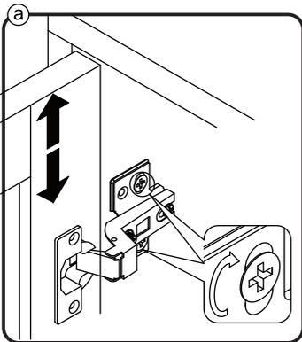
**EN** To adjust the door vertically loosen the screw as shown and move up and down as needed.
