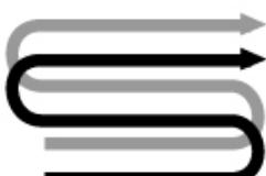
When preparing a seedbed, make the same path twice in the first row, then overlap half the width of the tiller on the rest of the passages.
