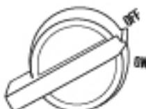
Position the starter switch on the side of the vehicle to 'ON'.
