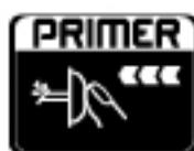
Press the 'Primer' button located under the choke lever 2/3 times until fuel can be seen flowing into the transparent pump.
