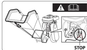
Warning! Emergency stop. Make sure the cable is properly connected
