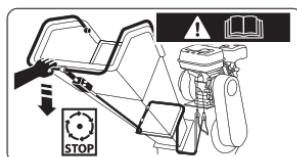
Warning! Emergency stop. Press the kill switch to activate it
