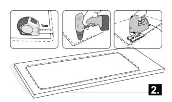
Draw another line 10mm inside the first line. cut a hole in the bench top following this second, inner, line. (if the manufacturer has included a pattern in the package, then use the pattern to cut the hole in the bench top).
