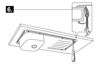
Tighten the screws of the anchor braces (with a hand screwdriver), to secure the sink in place.
