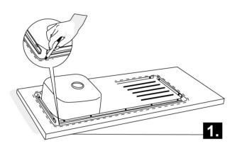
Place the sink upside down in the position where it is to be installed, and trace the outline of the sink on the bench top with a pencil.
