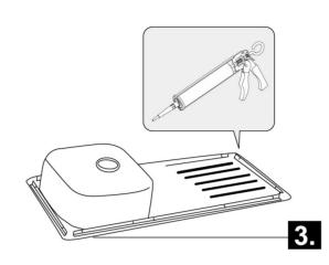
Adhere the rubber bench seal around the under side of the edge of the sink, being careful to lay it smoothly (without ridges).
