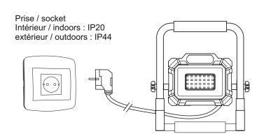
**EN.** 1. Loosen the two sides of the structure 2. Hold the foot and adjust the position floodlight then tighten the two sides
