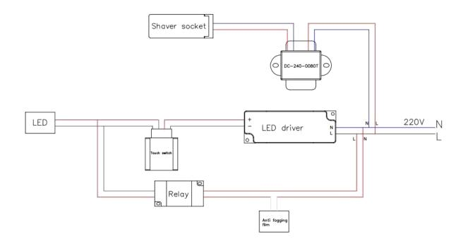
CDC3: Models with anti-fog/ sensor switch/ shaver socket/digital clock
