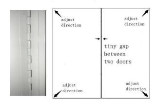
2.4.2.3 And if the gap is still not good after adjustment, then please hang the cabinet on the wall and do the adjustment as 2.4.2.2 again .
