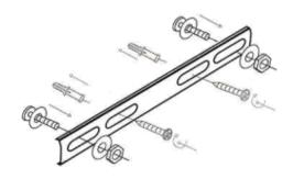
**Step 4** Fix the first frame with screws.
