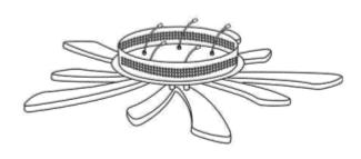
**Step 7**Connect the wires into theceiling electric wire.
