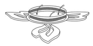
**Step 7**Connect the wires into the ceiling electric wire.
