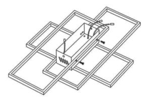
Connect the wires into the ceiling electric wire.
