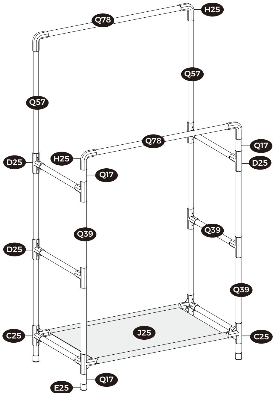
**EN** Insert the pipes into the bottom of the connectors, and then assemble the fabric cover.
