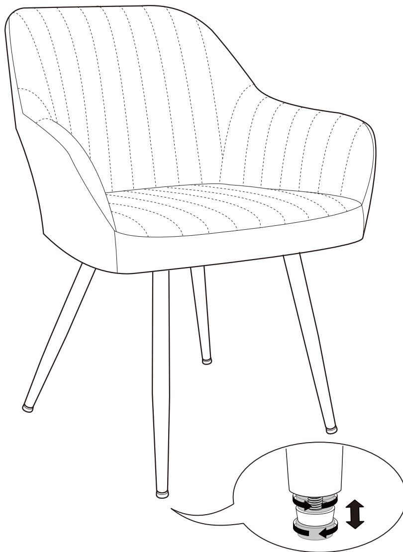
**EN** Screw in the adjustable feet to keep the chair balanced.
