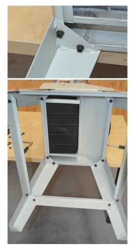
Leave all nuts and bolts finger tight until you have finished assembling the stand. Lay the machine on its back and bolt the four legs to its base, using the M6 x 10mm cap head bolts.
