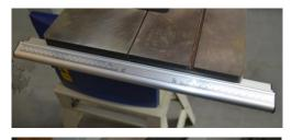
Offer up the fence rail so that the four slots slide over the shafts of the bolts and then tighten the wing bolts.
