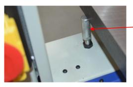
This special bolt sets the angle of the table for 90° cuts. When the edge of the table is resting on it, the blade should be perpendicular to the table top. If necessary this bolt may be loosened and an adjustment made.
