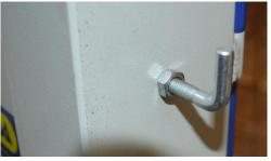
Screw a nut onto the push stick hook and screw this into the tapped hole high up on the left hand side of the saw. Lock it into position with the nut.
