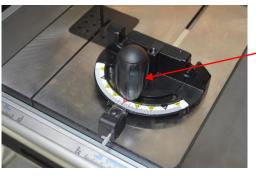
Slide the mitre fence into one of the T-slots in the table.
