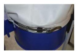
Feed the end of the collector bag clamp through the slit at the bottom of the cloth filter bag. Keep feeding it around the rim of the bag until it emerges from the other slit. Secure the clamp, by engaging the latch as shown.
