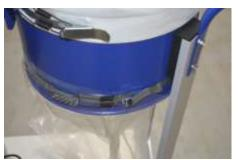
Slide the open end of the plastic collection bag over the bottom of the collector body. When working on your own, temporarily secure the bag in place with three pieces of sticky tape. Fit the second bag clamp around the plastic bag, as shown.
