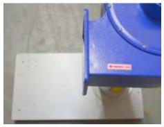
If necessary, twist the motor assembly so that the face of the outlet is parallel with the end of the base plate. Tighten the three fixing bolts.
