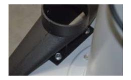
Bolt the floor sweep attachment onto the base plate using two M8 x 12mm hex head bolts and washers.
