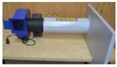
Position the base plate and column as shown. Insert the lower end of the motor into the column and fix it loosely with two M6 x 10mm hex head bolts and M6 washers. These screw into the tapped holes that can be found in the three lugs on the end of the motor .
