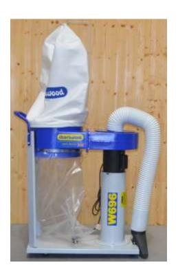
In addition to its function as a normal dust extractor, this machine may be used as a floor sweeper. This works best on a smooth floor.
