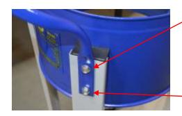
Take one M8 x 44mm hex head bolt, add a washer and push it through the upper hole of the handle, the collector support and the spacer block. Screw it a few turns into the threaded hole in the collector body. Do the same with the upper hole on the other side of the handle.
