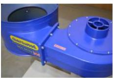
Locate the rubber gasket and place it between the collector body and the fan housing.
