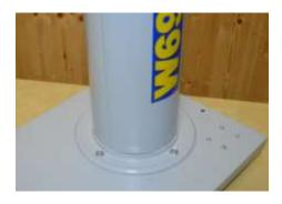
Invert the base so that it is standing on its castors. Rotate the column so that one of the slots in the top end of the column is aligned to the centre of the short side of the base plate.
