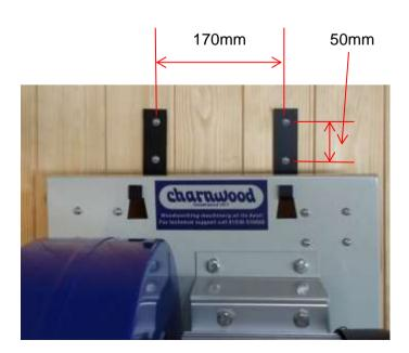
Two wall brackets are supplied in case you wish to wall mount the extractor. Attach these to a suitably strong wall using appropriate fixings.
