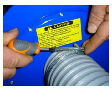
Connect the flexible hose to the dust hood and the extractor using the hose clips supplied.
