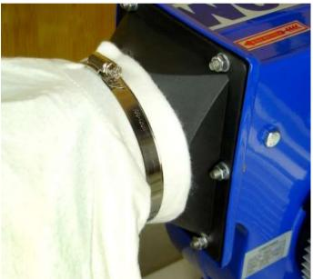
Fit the dust collection bag over the round outlet and secure it in place with the jubilee clip supplied.
