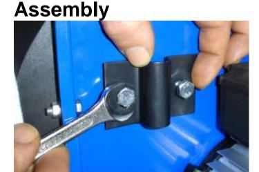
Attach the mounting bracket to the extractor fan housing using the two bolts provided.
