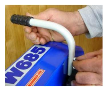
Fix the handle to the fan casing using the two M6 bolts supplied.
