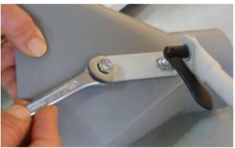
Attach the adjustable bracket assembly to the dust hood using the bolts, nuts and washers fitted to the hood. Ensure that the heads of the bolts are inside the hood and the nuts/washers outside.
