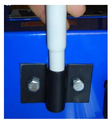
Insert the reduced end of the support arm into the mounting bracket.
