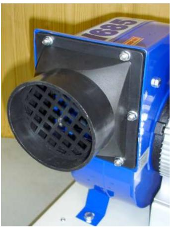
Fit the plastic adapter over the bolts and secure with washers and nuts. Add the remaining four bolts. Tighten the nuts when all six bolts are in position.
