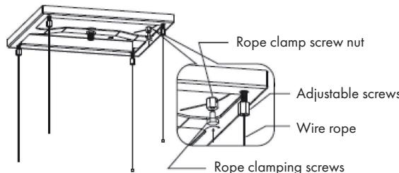
6. Drill 8 mounting holes on the ceiling corresponding to the 8 round holes on the hanging board and fix the hanging board to the wooden ceiling with 8 countersunk screws (ST6\* 40 mm) (see image 4). If the ceiling is made of concrete, you must drill 4 mounting holes corresponding to the 4 holes on the hanging board and use four countersunk screws( $\varnothing 6 * 60$ ) to fix the hanging board to the ceiling.
