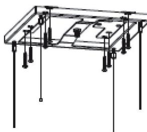
7. Attach the 4 wire ropes to the cover and use the locking nut to secure the cover to the suspension board. (See image 5). Note that the hole for the power cable on the cover plate should be in the same direction as the hole for the power cable on the cooker bonnet.
