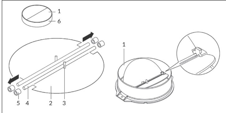
If you have an air outlet to the outside, the cooker bonnet can be connected via an extraction duct (enamel, aluminium, flexible pipe or non-combustible material with an internal diameter of 150 mm) as shown on the right.
