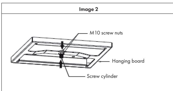
5. Attach the 4 adjustable screws to the hanging board, turn them to the right length and not too tight. The height of the 4 screws is basically the same. Pass the 4 wire ropes through the 4 adjustable screws, calculate the length of the wire rope according to image 1 and mark the length on the rope. Use the 4 rope clamping screws + nuts to fix the 4 ropes at the marked points. Make sure that the 4 ropes are of equal length (see image 3).
