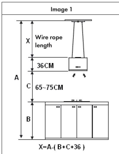
3. The ceiling must be able to support a weight of at least 120 kg and the thickness of the ceiling must be  $\geq 30$  mm.
