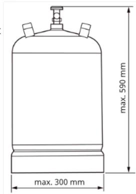
This gas barbecue can only be used with a gas bottle which does NOT exceed a **maximum height of 590 mm** and a **maximum diameter of 300 mm**. If there is no suitable trolley or base cabinet is not available for your gas bottle. The gas bottle must be placed at a minimum distance 60 cm from the barbecue.
