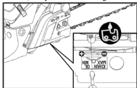
The setting screw for the oil volume is on the underside of the chainsaw.
