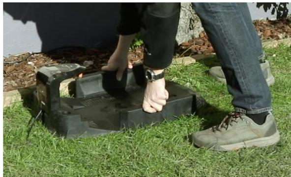
The charging station must be placed on a firm, level surface with the "IN" arrow on the charging station pointing towards the work area.
