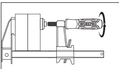
④ Rotate the handle clockwise to make sure the workpiece is firmly secured.
