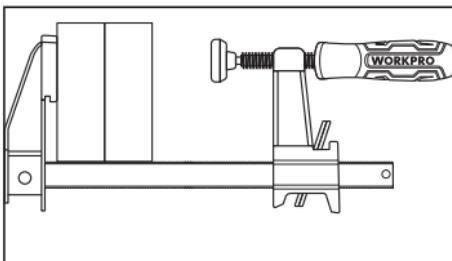
② Insert the workpiece into the open jaws of the clamp.
