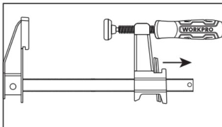
① Press the quick-release trigger and move backward to necessary width then release the trigger.
