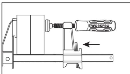
③ Press the quick-release trigger and slide forward along the bar to clamp the workpiece.
