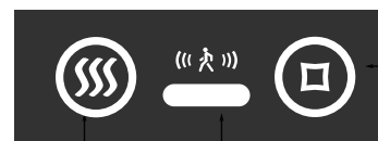
① Demister Switch & Movement sensor function ② Sensor display screen ③ Light Switch & Brightness Adjustment
