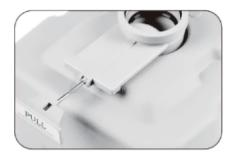
Step 2. Open the sealing diaphragm handle to fully open the partition and keep the lever open during use.
