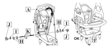
Step 5. Put on the iron shaft at the connection of the seat base and fix it with screws. The seat installation is completed.
