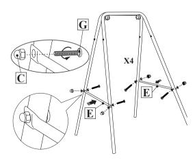
Step 2. Lock the C G screws on the E iron pipe as shown in the figure. The iron frame installation is completed.
