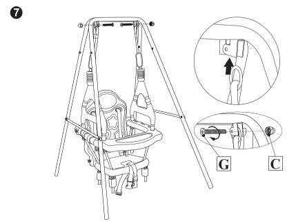
Step 7. Fix the seat with the rope on the iron frame with C G screws. The entire installation is completed.
