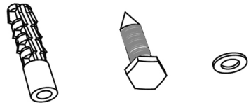
\phi 10 \times 50 anchor bolt, M8 \times 75 hexagon wooden screw, \phi 8 washer (x4 pcs)
