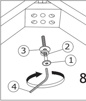
Tighten part (D) with part (A) completely after alignment is done.
