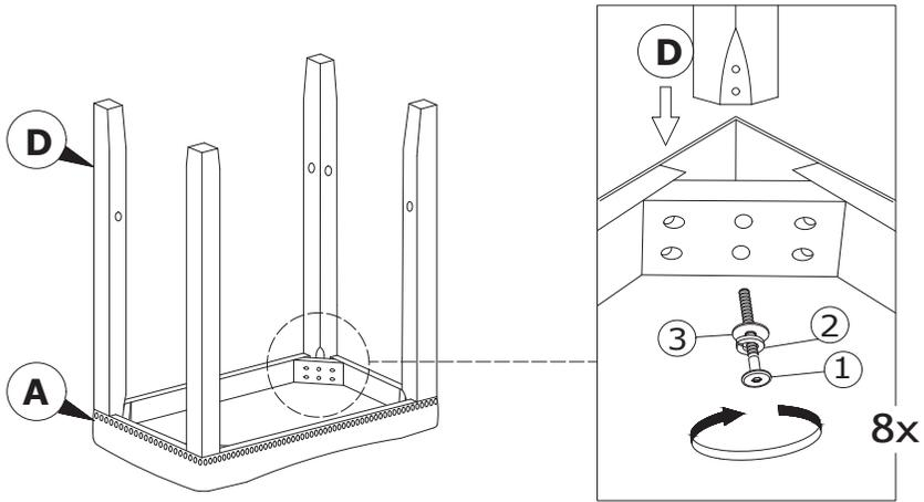
Do not tighten the hardware completely!
