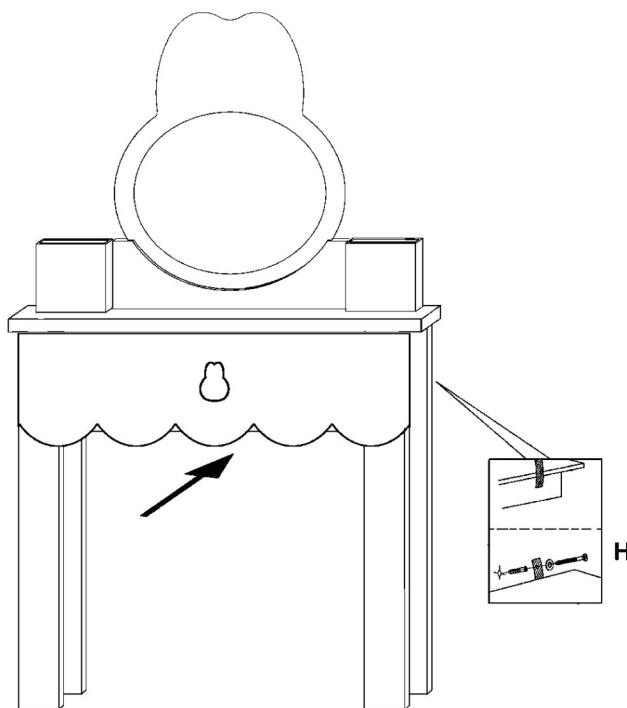
**EN:** Push the drawer (A) into the table body (E), and use the accessory (H) to fix the table to the wall to prevent it from tipping.
