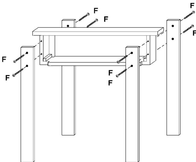
**EN:** Use screws (F) to pass through table legs (D) and fix them on 4 corners of the table.
