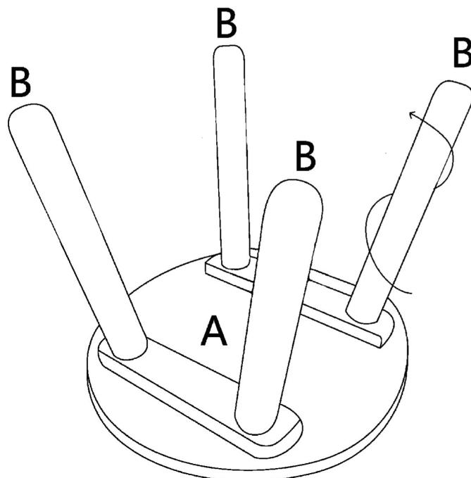
**EN:** Rotate to install the stool legs (B) to the stool body (A).
