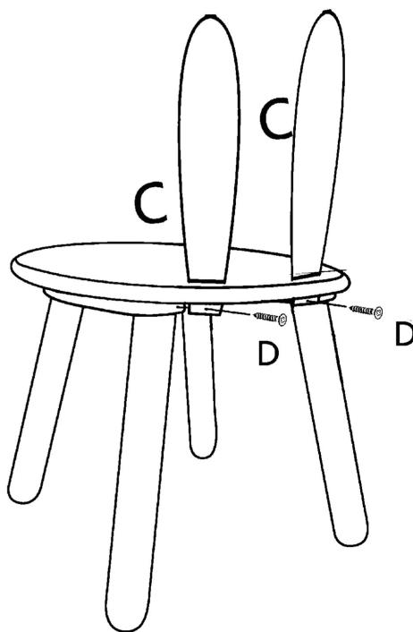
**EN:** Pass the part (C) through the stool and make screws (D) pass through the part (C) to fix the part (C) on the stool (A).
