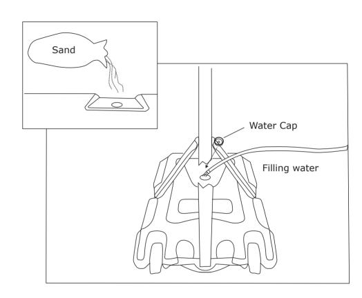
Filling the Base(S) with water or sand to keep steady.
