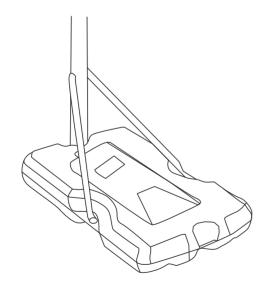
Fix the other end of Pole Brace(L1)&(L2)on two sides of Base(S) by Bolt Set (C1),(C2)&(C3) as shown.
