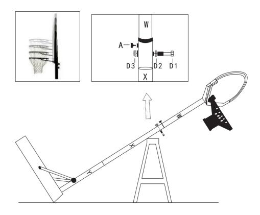
Insert the Top Pole (W) into the Middle Pole (X), adjust it to the desired height, and then fix it with the plastic knob (A) and bolt sets (D1), (D2) and (D3), as shown in the figure.
