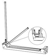
EN: Depress the release lever and rotate the leg until it clicks and locks into the open position.
