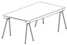
EN: When paired together with a second unit and properly joined by 45x90mm in support arms, a work table can support up to 454kg.
