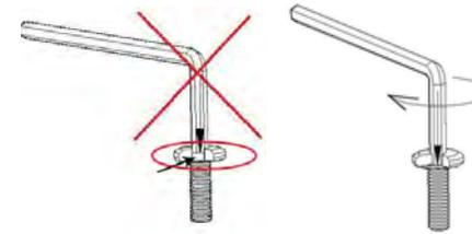
If you don't do that and slip out of the screw, the screw will suffer damage and it can cause the screw head to become round inside so that you won't be able to find grip with the hex key anymore. Round spun screw heads only result from this and aren't a reason for complaints.
