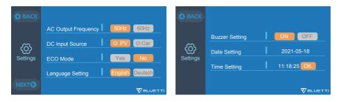
Note: Check all settings before first use. Please set the system date and time every 2 weeks. Voltage and frequency for reference: US: 120V/60Hz S EU: 230V/50Hz UK: 230V/50Hz AU: 240V/50Hz
