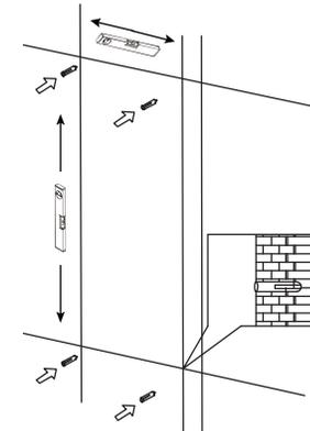
Mark the position of the screws on the wall, then drill four holes accordingly and tap the number G on the wall.
