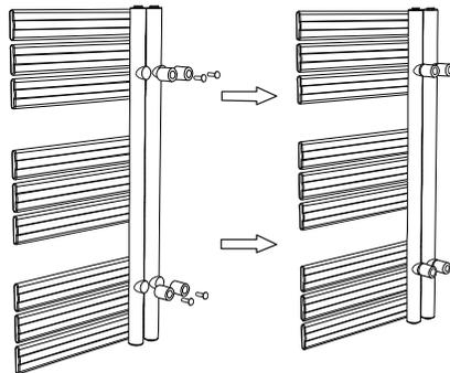
**Step 4:** Mount the radiator to the wall and tighten the Small Screws I in the brackets.
