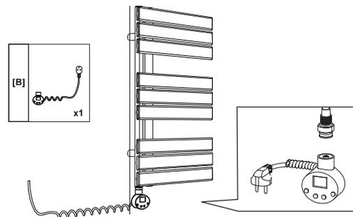
1. Ensure the heating rod pins align with the hole on the thermostat unit, then insert the pins securely
