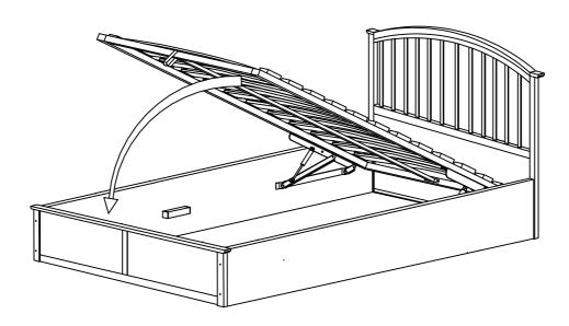
Lift with the strap (H10) and close with the strap. The strap should always be accessible. Take care not to lean over the bed when lifting, if the mattress is thin and light, the frame may rise quickly. The speed of closing will also depend on the weight of the mattress so always keep fingers well clear of the metal frame.
