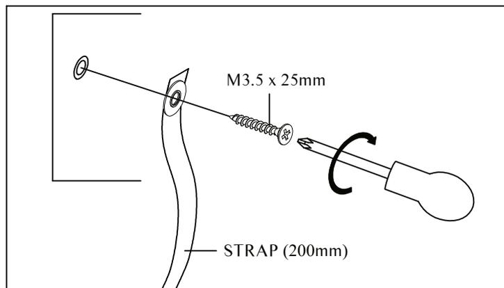
**NOTE:** Wall fixings are not supplied with this product as different wall materials require different types of fixing devices (such as Rawl plugs on bricks wall). You must use fixing devices suitable for the type of wall you intend to mount this product to. Please ensure that the head of any screw used has a diameter greater than the diameter of the mounting hole on the product and that the fixing is safe and secure before use.
