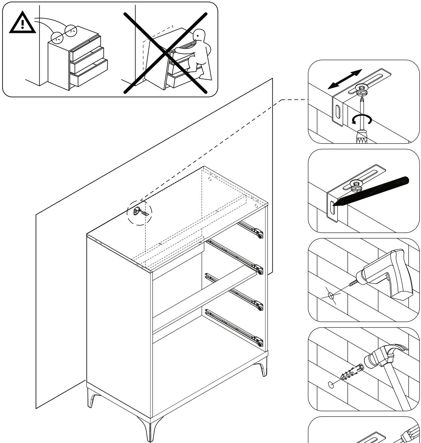
**NOTE :** Wall fixing are not supplied with this product as different wall materials require different types of fixing devices (such as Rawl plugs on brick work). You must use fixing devices suitable for the type of wall you intend to mount this product to. Please ensure that the head of any screw used has a diameter greater than the diameter of the mounting hole on the product and that the fixing is safe and secure before use.
