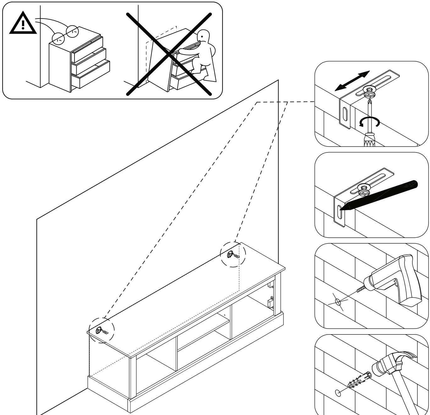
**NOTE :** Wall fixing are not supplied with this product as different wall materials require different types of fixing devices (such as Rawl plugs on brick work). You must use fixing devices suitable for the type of wall you intend to mount this product to. Please ensure that the head of any screw used has a diameter greater than the diameter of the mounting hole on the product and that the fixing is safe and secure before use.
