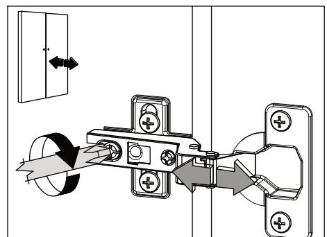
C. Front-to-back adjustment (Spacing Door Off Carcas) by slackening the hinge arm mounting screw
