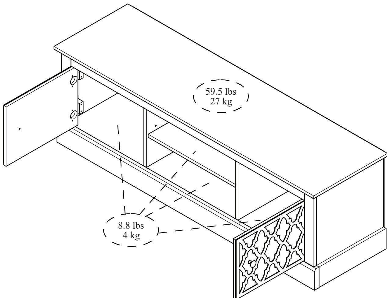
This unit has been designed to support the maximum loads shown. Exceeding these load limits could cause sagging, instability, product collapse, and/or serious injury.
