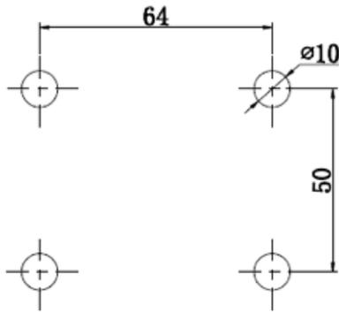
2. Place the anchors in the holes: with the help of a hammer, insert the 10mm anchors into the holes.
