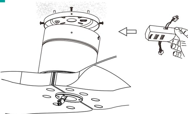
Hang the motor assembly and place the receiver in the holder,
