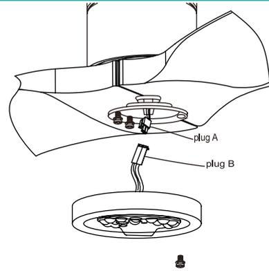
Remove the screws. Align the holes of the lamp base and rotate the lamp base clockwise to ensure the two screws seat firmly.
